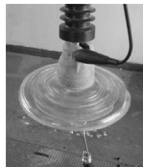
Fig. 22 – Insulator in test for verification of the capacitance.
