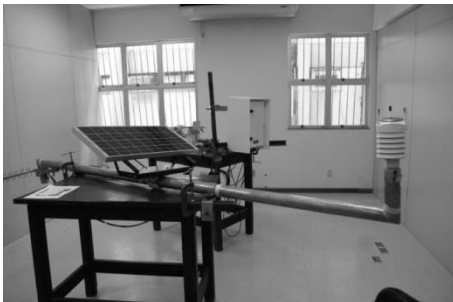
Fig. 30 – Remote Meteorological Station (EMR) in operation test.
