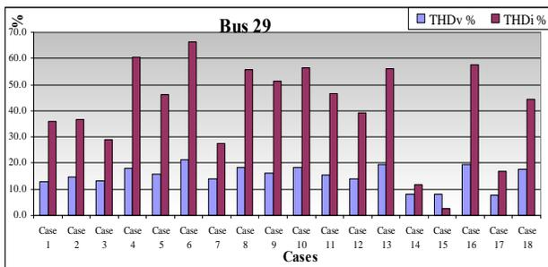
Fig. 14 Comparison for THDv and THDi at Bus 29 on different cases
