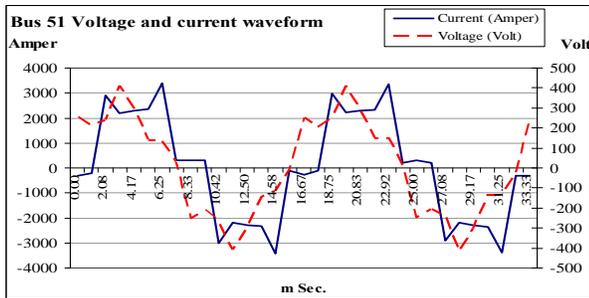
Fig. 7 Current and Voltage waveform at Bus 51
