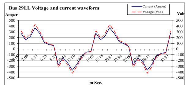
Fig. 5 Current and Voltage waveform at Bus 29:LL (Linear Load)
