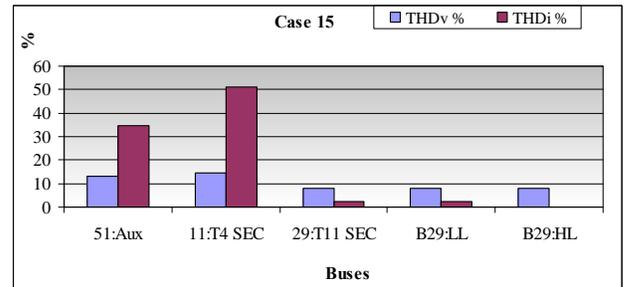
Fig. 11 Voltage and Current THD at Buse51, 11 & 29
