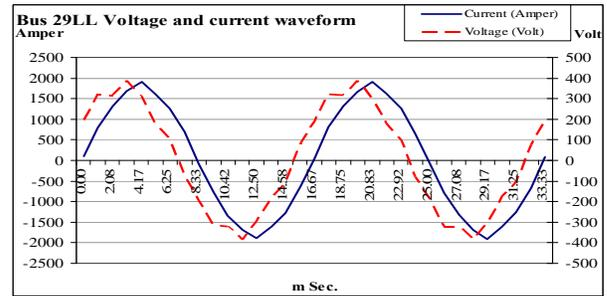
Fig. 10 Current and Voltage waveform at Bus 29:LL (Linear Load)
