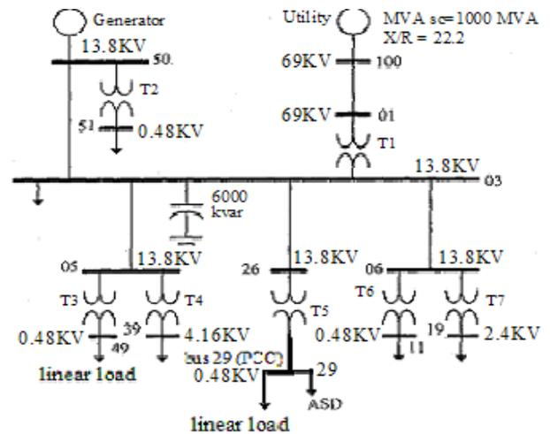
Fig. 1 The modified 13 buses (BIDS) Test system presented at [5]
