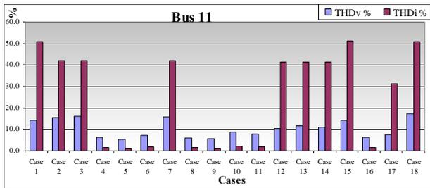
Fig. 13 Comparison for THDv and THDi at Bus 11 on different cases
