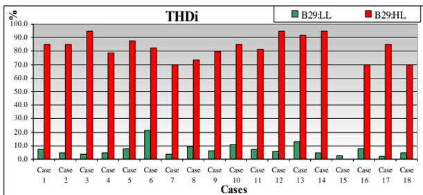
Fig. 15 Comparison THDi at linear load and nonlinear load of Bus 29 for different cases
