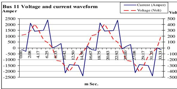
Fig. 8 Current and Voltage waveform at Bus 11
