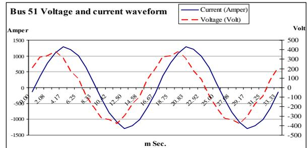
Fig. 2 Current and Voltage waveform at Bus 51
