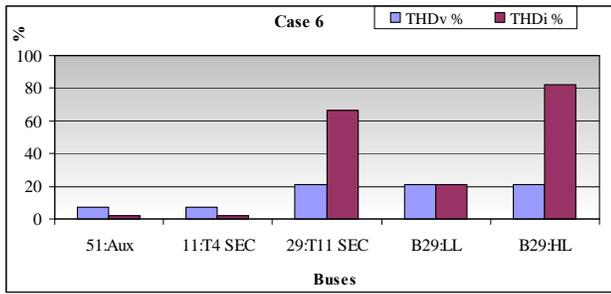
Fig. 6 Voltage and Current Total Harmonic Distortion at Buse51, 11 &29
