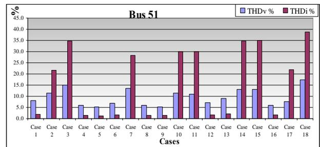
Fig. 12 Comparison for THDv and THDi at Bus 51 on different cases
