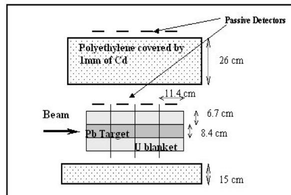
Figure 2. A cross-section of the Pb/U-blanket assembly.
