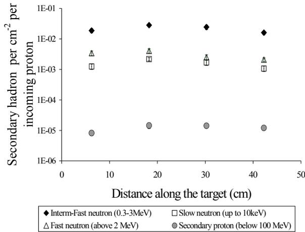
**Figure 4.** Hadrons production yield over the Pb(U-blanket) target irradiated by a relativistic proton beam with energy 1 GeV.
