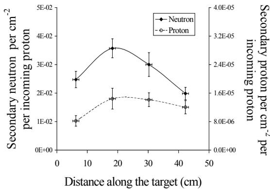
**Figure 5.** Secondary hadron spatial distribution measured over the Pb(U-blanket) target irradiated by a relativistic proton beam with energy 2 GeV.
