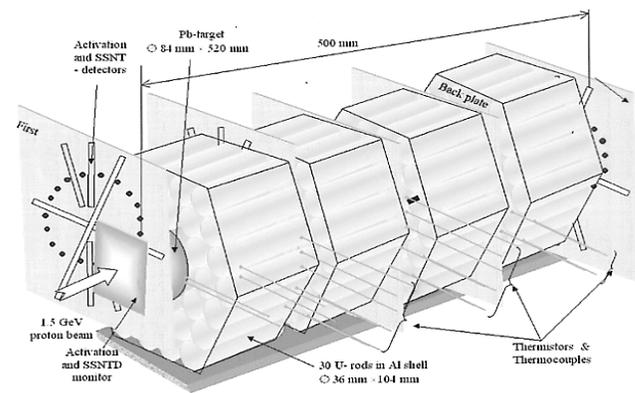
Figure 1. The “Energy plus Transmutation” set-up.
