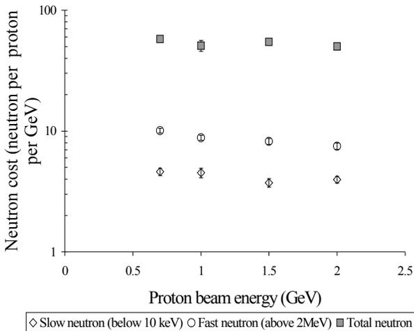
**Figure 6.** The “neutron cost” of secondary neutron production using relativistic proton beams.
