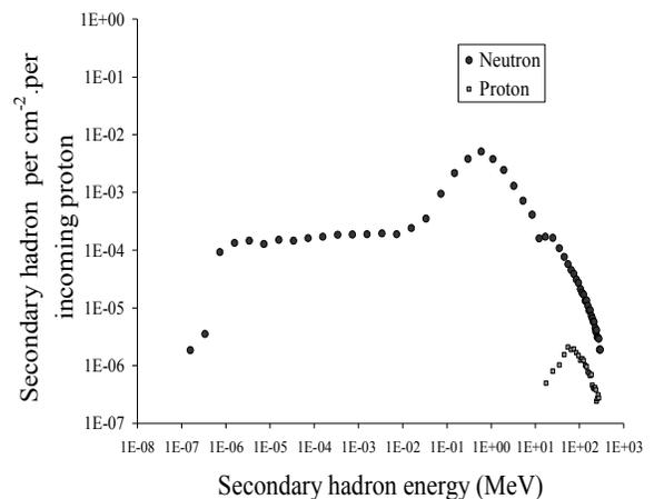
**Figure 3.** Monte-Carlo simulations of the energy dependent secondary hadron fluence using the Dubna Cascade Model for the Pb (4-section U-blanket) target irradiated by a relativistic proton beam.
