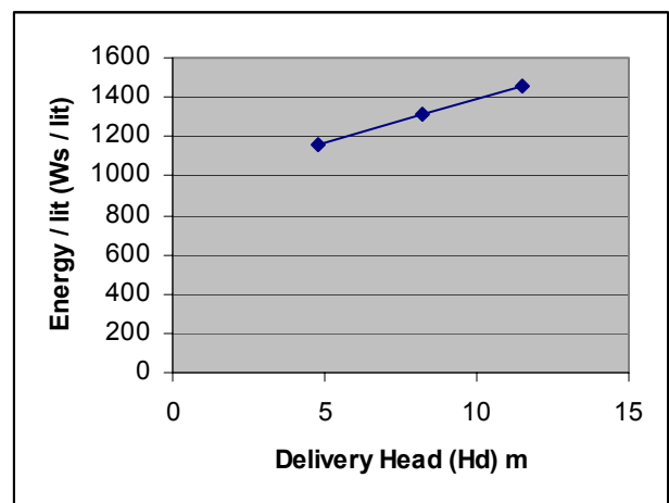
Fig. 3 Energy Consumed by Pump in 2 storied building at Hs = 1.2 m
