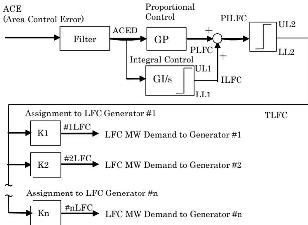
Fig. 2 Simplified model of load frequency control
