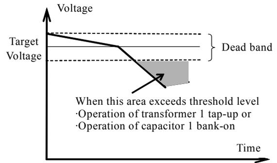
Fig. 3 Simplified model of local voltage control (voltage control based on time integration of voltage deviation at load node)
