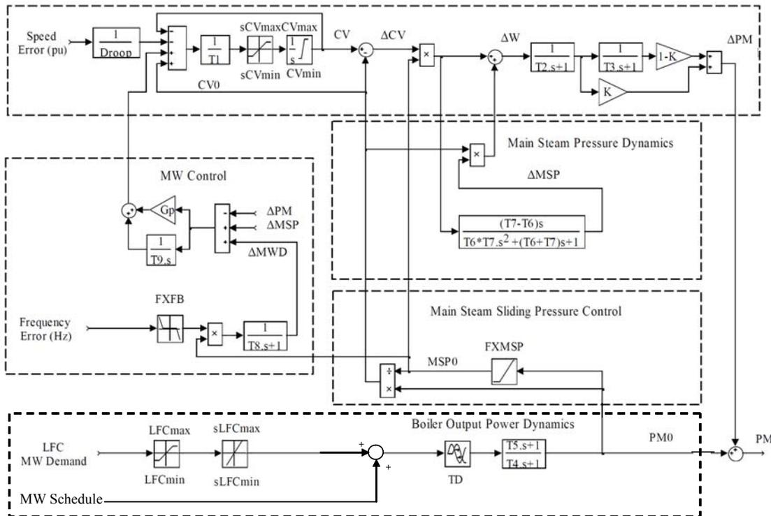
PM0: Slow component of PM ΔPM : Fast component of PM (PM: Turbine mechanical power)
