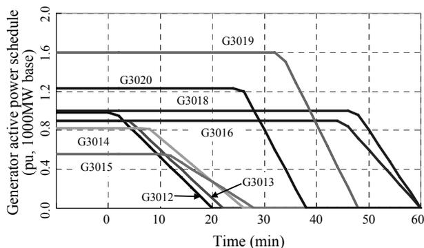
(b) Change in MW schedule of generators with output power regulation (8 generators)
