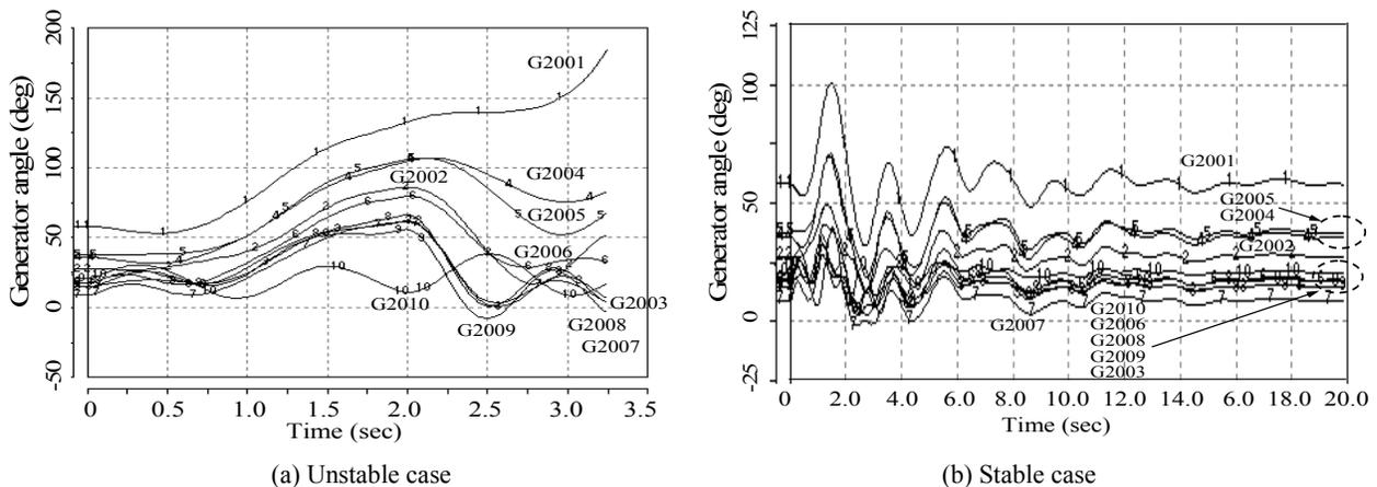
Fig. 6 Angle stability simulation results of proposed program (1cct-3LG fault at position A in Fig. 5)
