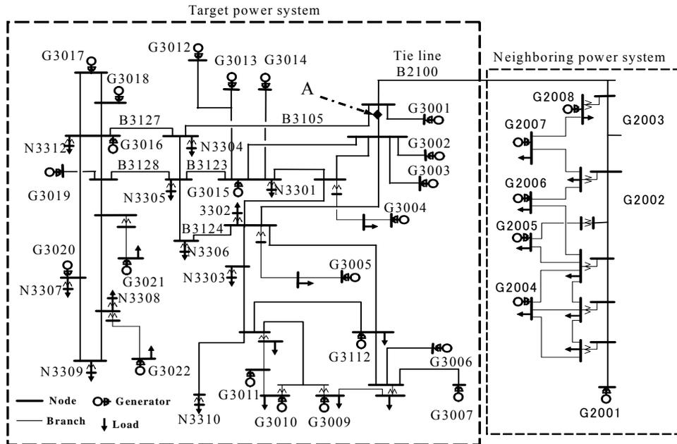
Fig. 5 IEEJ EAST-30-generators test-power system [6]
