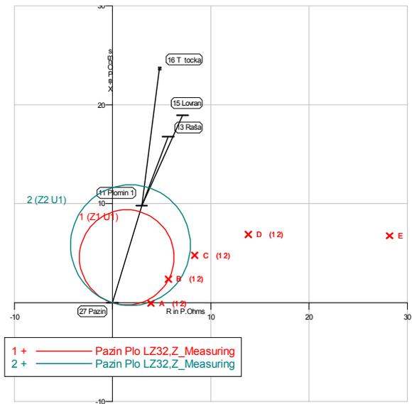
Figure 6 Tripping Characteristic of the Relay LZ32 in Pazin – R=2.5Ω, New System Configuration
