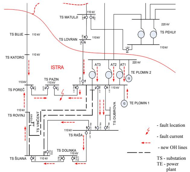
Figure 1 Analyzed Part of TSO Rijeka With Fault Current Distribution
