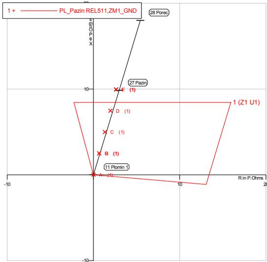
Figure 4.a Tripping Characteristic of the Relay REL511 in Plomin – R=0Ω
