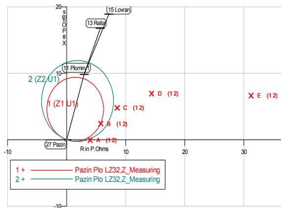
Figure 5.c Tripping Characteristic of the Relay LZ32 in Pazin – R=2.5Ω
