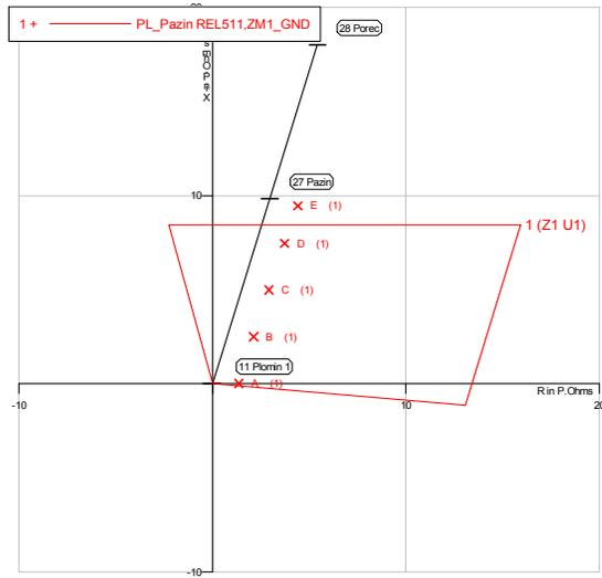
Figure 4.c Tripping Characteristic of the Relay REL511 in Plomin – R=2.5Ω
