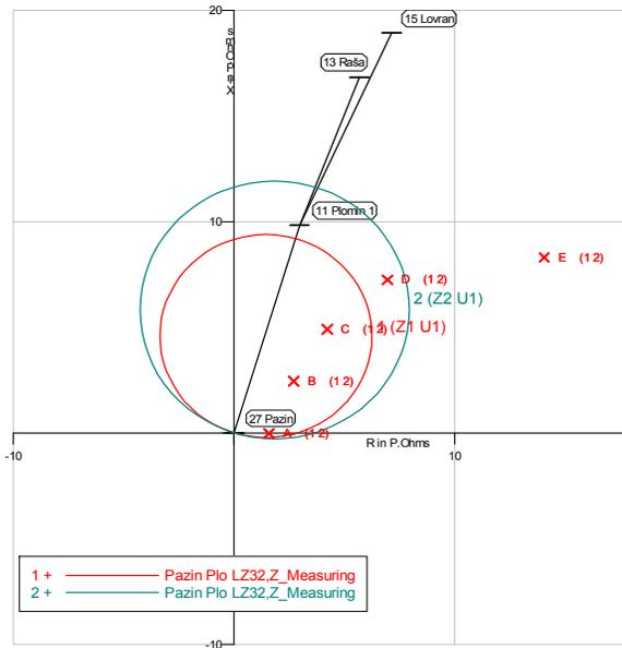
Figure 5.b Tripping Characteristic of the Relay LZ32 in Pazin – R=1Ω
