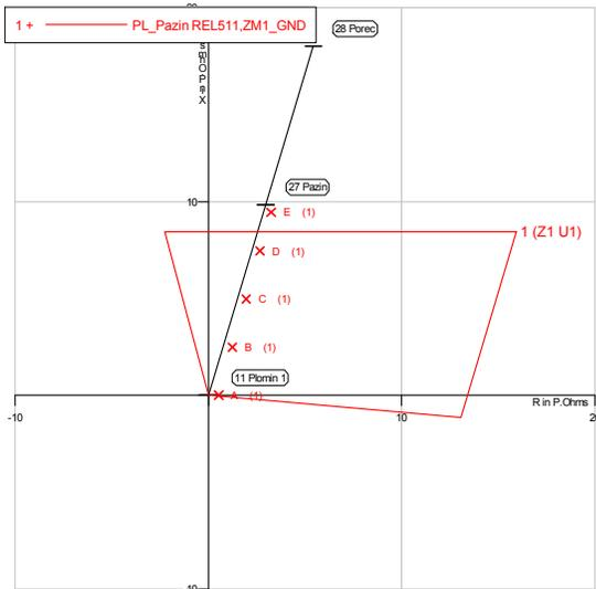
Figure 4.b Tripping Characteristic of the Relay REL511 in Plomin – R=1Ω
