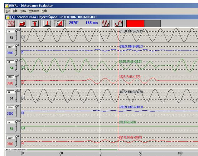
Figure 2 Oscillogram of Currents and Voltage During Single – Phase to Ground Fault on the Line Raša - Šijana
