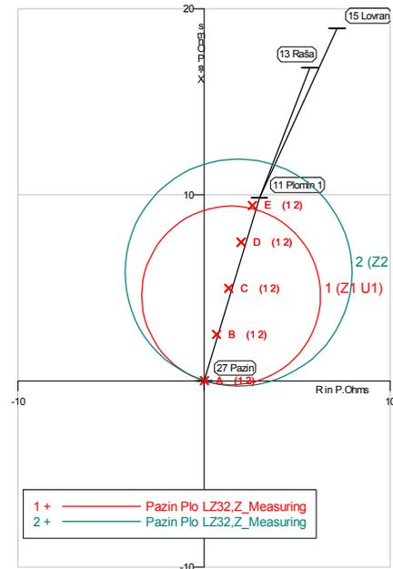
Figure 5.a Tripping Characteristic of the Relay LZ32 in Pazin – R=0Ω
